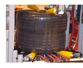
The conveyor units receive and position the products. The lifting and turning unit is raised and the hold-down device is lowered. The wrapping process is carried out. Afterwards, the packaged product is transported out of the machine and the new product is received.
