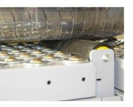
This lifting unit is raised during the wrapping process! It is possible to freely turn the tyres and fix them in place using two fingers. The film does not catch in the ball rollers during the wrapping process.
