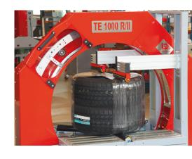
This lifting unit is raised during the wrapping process! The tyres are turned manually or automatically. The automatic film holder and cutter neatly places the end of the film on the bottom of the package.
