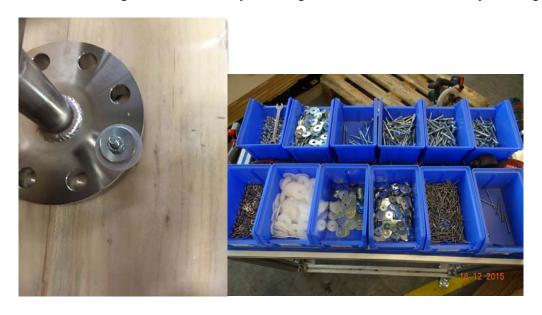
Material of Screws are ABC-Spax-S, steel,  $4.5 \times 50$  and ABC-Spax-S, steel,  $4.5 \times 70$ . All screws, which are used for packing are of galvanized steel. Generally for screwing also washers are used to tighten and stabilize the goods,
