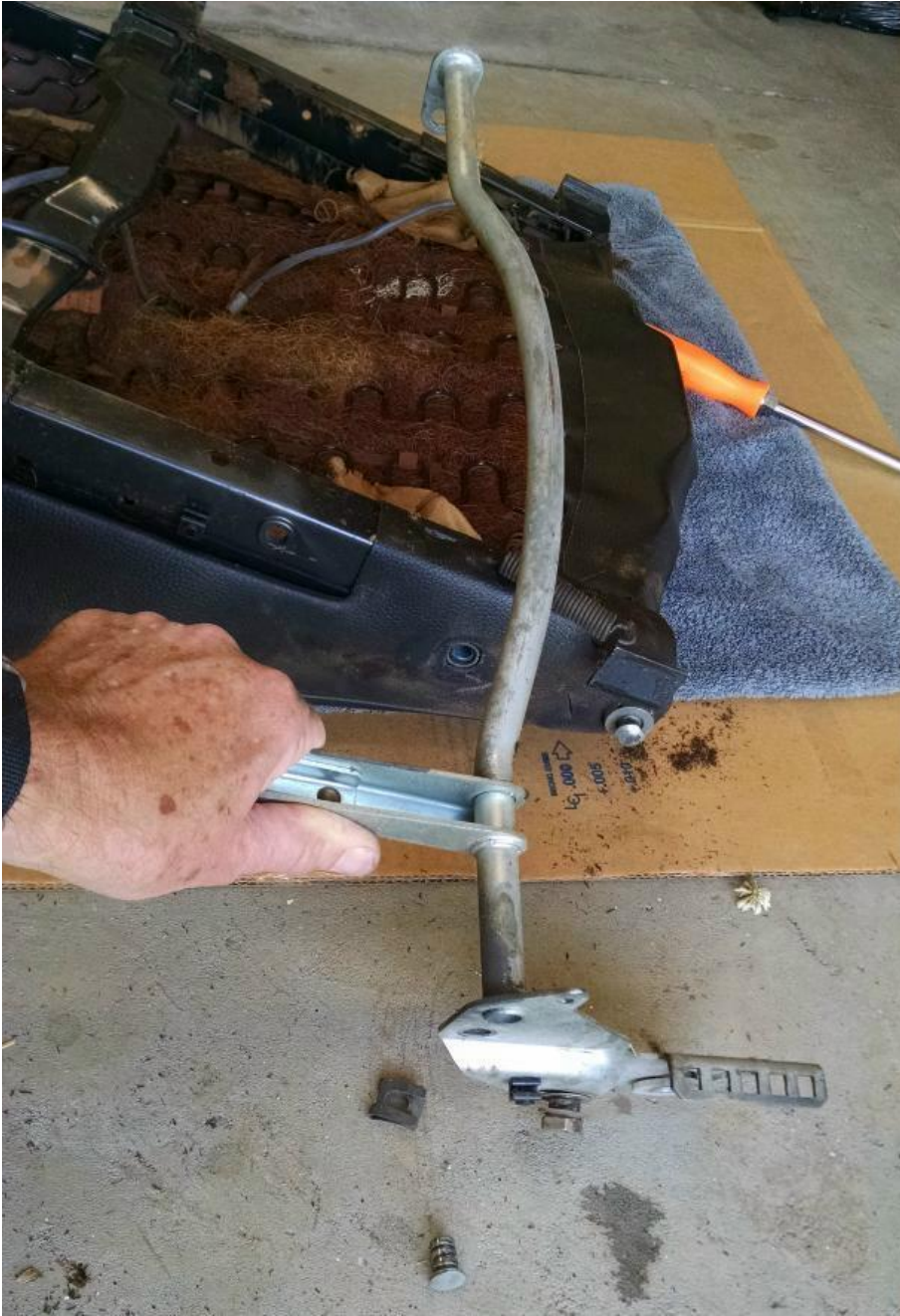
13. Remove adjuster lever from seat. (there are 2 main parts, plus one separate stud and the two Tinnerman clips)
