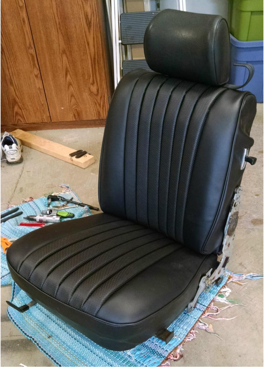
45. Finished seat ready to slide the adjuster rails back on.
