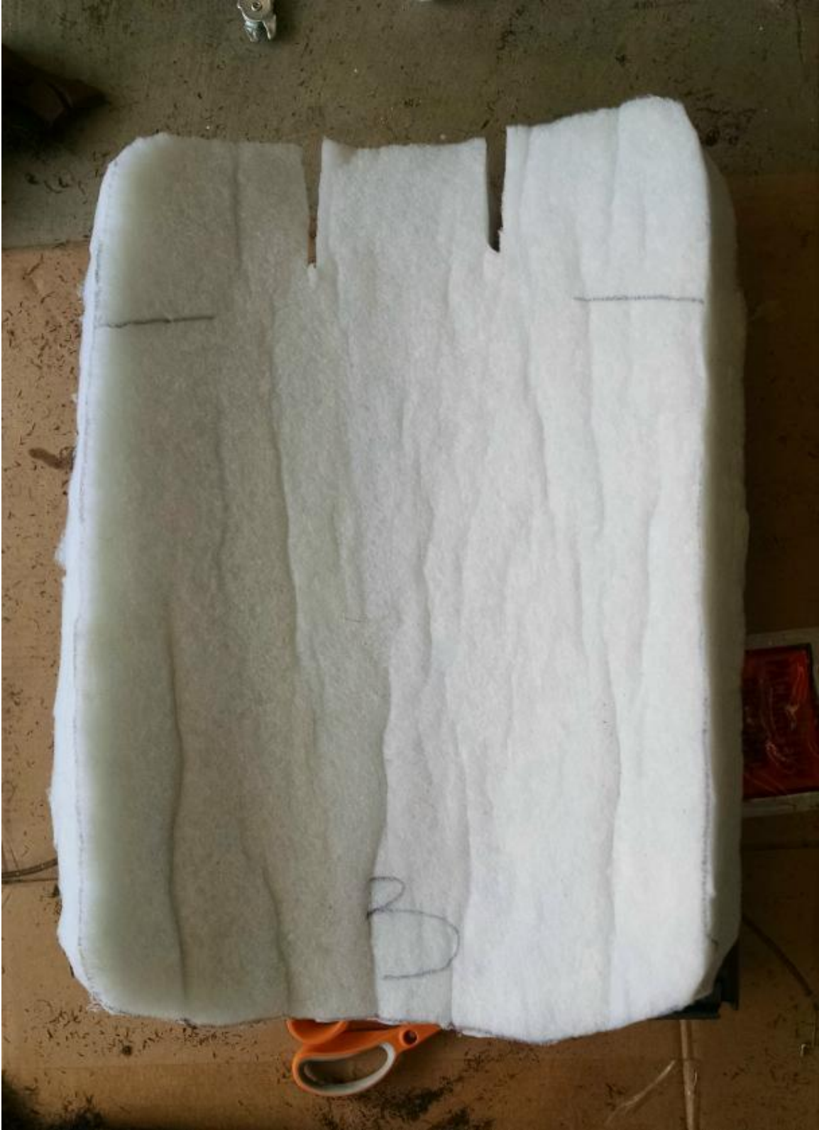
38. Here's the new pad, with notches cut out at the top where the headrest posts will have to pass through.
