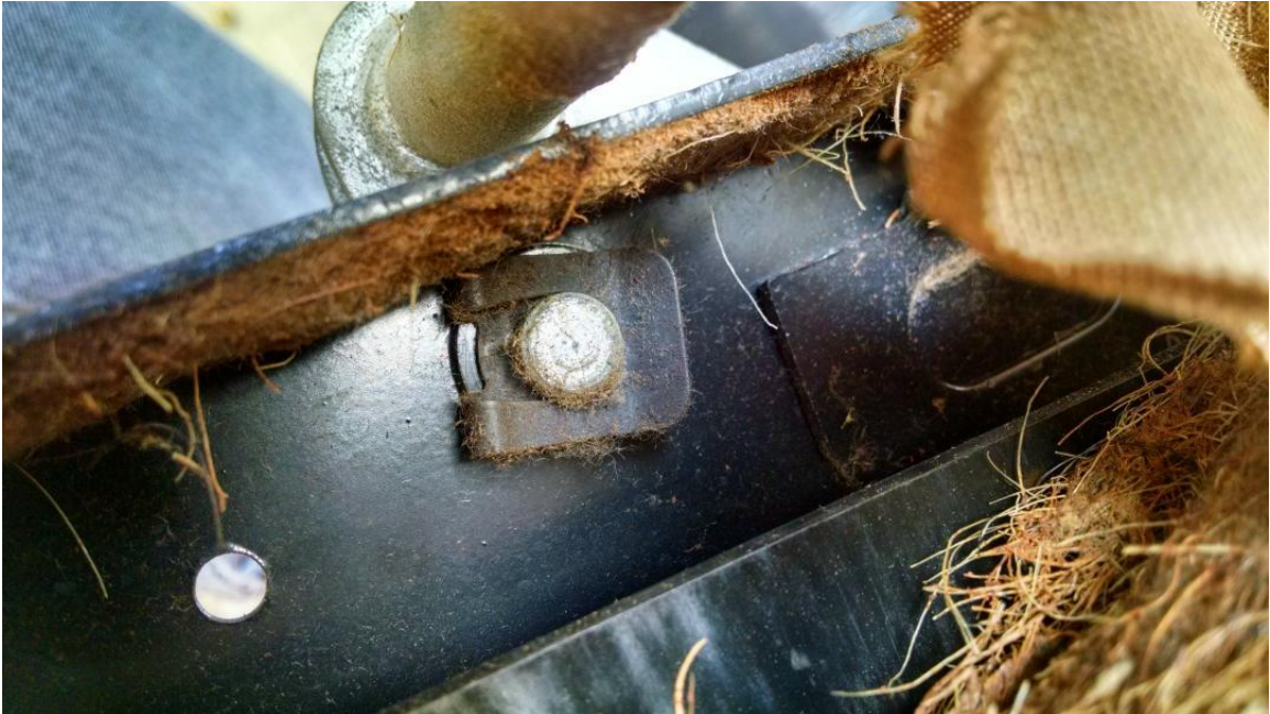
12. Remove Tinnerman clips on both sides of frame to release adjuster lever assembly.
