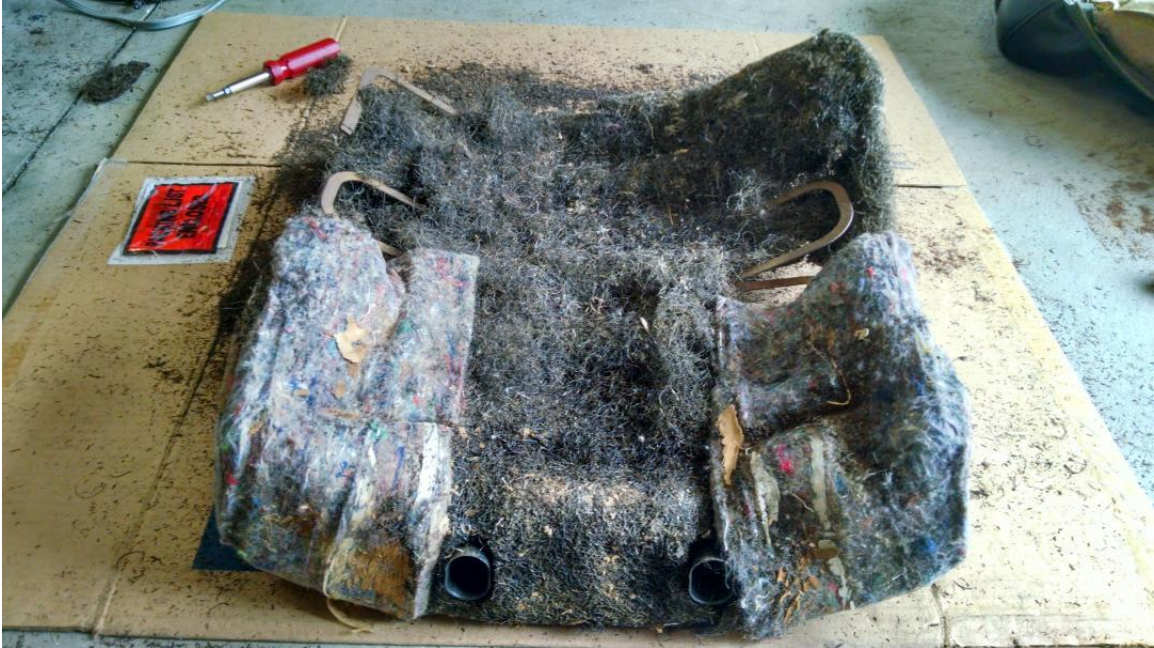
36. Here's what it looks like under the skin. Not much here worth saving, not even enough of the pad left to use as a template to cut the new pad.
