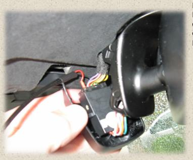
I saw <u>these instructions</u> on the Corvette Forum, and hope it helps anyone that wants to install and provide power to a Radar detector using the Blendmount mirror bracket! There is some concern that this may create issues for the cars' computer, but I haven't heard of anyone on the forum having trouble!
