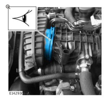
Check the throttle intake manifold to cannister seal for signs of oil leakage from the o-ring seal.
