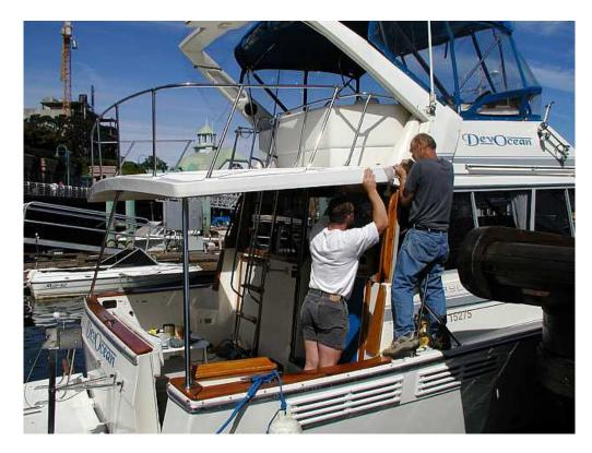
5. Align companion way opening in hardtop with existing ladder opening in cabin top. Make sure hardtop is not twisted to port or starboard. Sight down hardtop sides and make sure hardtop is square to cockpit sides. The opening in the hardtop for the ladder should be as far forward as possible .Approximately 5 to 51/2 inches of the hardtop flat flange should rest on the existing cabin roof. Clamp in place. Re check alignment.
