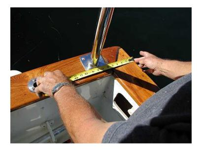
b. Align the center of the port stainless steel stanchion tube with the 8 inch mark.
