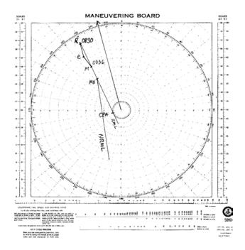
Step 7: Parallel the NRML from  $M_x$  to M (not to e, not to r, to M!) Draw the paralleled line away from M.
