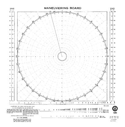
Step 2: Plot the first (0830) contact using the 1:1 scale (the ten concentric circles on a Maneuvering Board each represent 1 mile in length) at a bearing of 329° and range of 9 miles. Label it **r**.
