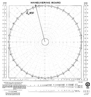
Step 3: Locate  $\mathbf{e}$  on the plot. Set dividers for the distance our vessel will travel in the interval of the plot -- in this case, 6 minutes at a speed of 15 knots is 1.5 miles. Parallel the course line (345°) over to  $\mathbf{r}$  and draw it in <u>backwards</u>, away from  $\mathbf{r}$ . [Remember the course is <u>from</u>  $\mathbf{e} \rightarrow \mathbf{r}$ .] Label this position  $\mathbf{e}$ .
