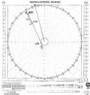
closest point (a perpendicular) on the RML is the CPA (closest point of approach). In this case, the CPA is about <u>one mile</u>. Measure the length of  $r\rightarrow m$  to find the contact's relative speed. Here it is approximately 30 knots.
