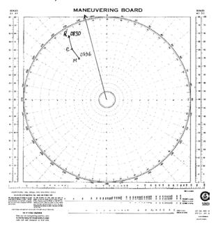
Step 5: Draw a line from **r** through **m** and past the center of the maneuvering board. This is the line of relative motion (RML). The distance from the center of the plot (our vessel) to the
