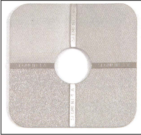
Fig. 3: Visual comparator to determine profile height created by abrasive blasting with metallic grit.
