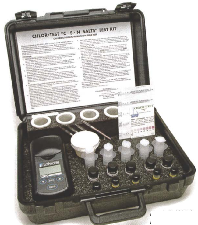
Fig. 1: Field kit for measuring salt content of abrasive Courtesy of Elcometer Instruments Ltd
