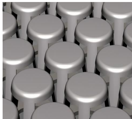
Fig. 2. Exploded view of tripod umbrellas fitted on the tray plate.
