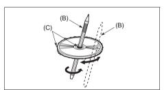
New discs may have some roughness around the edges. The unit may not work or the sound may skip if such discs are used. Use a ball-point pen (B), etc. to remove the roughness (C) from the edges of the disc before inserting it into the unit.
