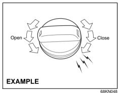
To remove the fuel filler cap:
