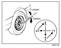
Tightening torque for wheel nut 85 Nm (8.7 kg-m, 62.7 lb-ft)
