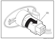
2) Turn the bulb holder (2) clockwise and pull it out from the light housing.
