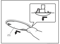
1) Remove the light housing (1) by sliding to left with your finger.
