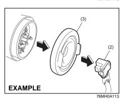
1) Open the engine hood. Disconnect the coupler (2). Remove the sealing rubber
