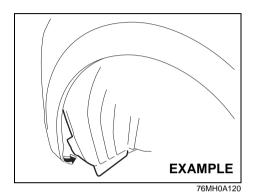
3) Open the end of the cover inside the fender.
