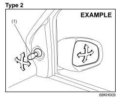
You can adjust the outside rear view mirrors by hand with the knob (1) located on the driver's or front passenger's door panel.
