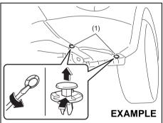
2) Remove the clips (1) by prying it off with a flat blade screwdriver as shown in the illustration.
