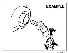
4) Disconnect the coupler by pushing the lock release. Turn the bulb holder counterclockwise and remove it.
