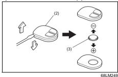
(3) Lithium disc type battery: CR1616 or equivalent
