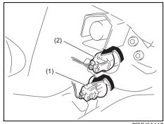
1) Open the engine hood. To remove the bulb holder of the front turn signal light (1) or the front position light (2) from the light housing, turn the holder counterclockwise and pull it out.
