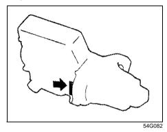
The engine serial number is stamped on the cylinder block as shown in the illustra-
