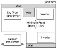
Separate transformer arrangement
