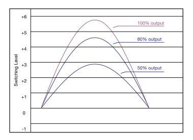
Patented design of cyclic switching rotates the cell sequence. This ensures equal heating and stress on each component of the cell. This method increases the overall reliability of the drive.
