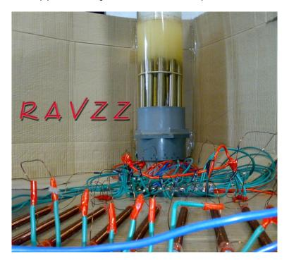
Above is a picture of the multiple bifilars Ravi tried on the WFC. These were connected to each pipe individually. Diode used 1200 V 40 Amps. Solid core length 8" wound with 0.711 mm conductor end to end. The generation increased by approximately another 10cc of gas for a 20 second period compared to regular wound inductors. This works on efficiency!! Need to try out other combos to see if it can increase some more.
