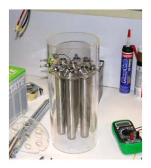
If using the sealed copper wire option, the ends of the copper wire needs to be sealed with high temperature heat resistant silicone sealant and should not contact water, as this generates a lot of greenish brown muck. Therefore put silicone sealant or automotive gasket silicon sealant all over it so that the water doesn't touch any of these parts. Then use the sealant over the exposed copper wire.
