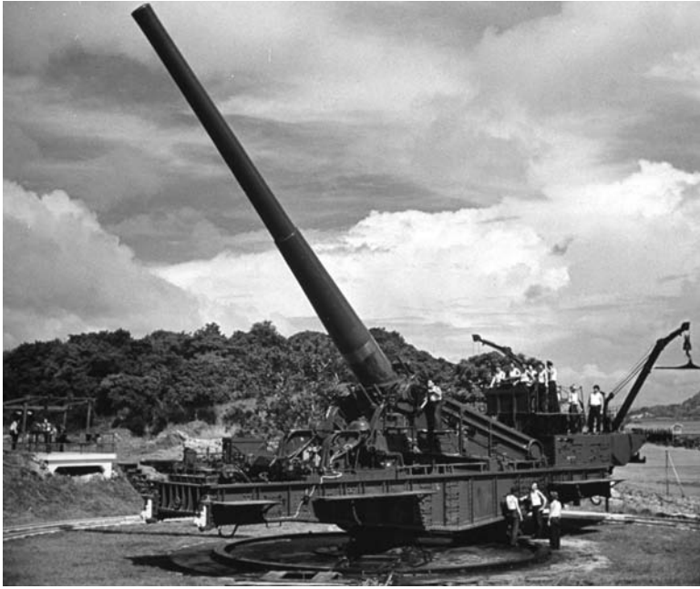
One of two 14-inch railway guns defending the canal. A rarity in the American arsenal, they were well suited for Panama because they could shift from one coast to the other as needed and occupy prepared positions.
