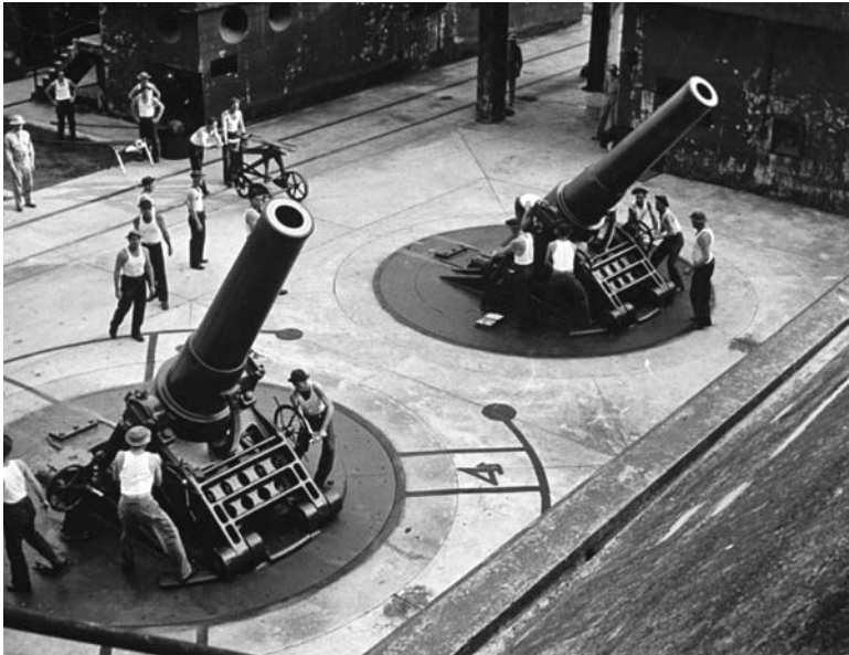
Crews man a pair of 12-inch mortars, probably at Fort Grant on Flamenco Island. There were 28 of these among the 51 coast defense weapons of 12 inches or greater at Panama.
