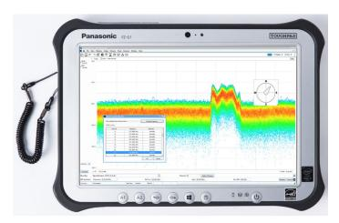
Tektronix offers the Panasonic FZ-G1 tablet controller as an option to the RSA306B and RSA500A series USB spectrum analyzers and as a standalone unit. When purchased from Tektronix, the FZ-G1 includes preloaded SignalVu-PC software, with custom-programmed display settings and front-panel buttons to optimize the SignalVu-PC experience. In addition, Tektronix has tested the FZ-G1 to ensure that the specified real time performance of all USB spectrum analyzers is met with this configuration.
