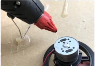
Glue motors to end of launcher.
