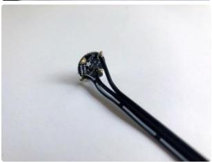
If you're using more than one NeoPixel, you'll want to solder two wires into the + and - pads, so you can pass power to the next pixel on down the line. Solder a wire from OUT on your first pixel to IN on the next pixel in the series, and so on.
