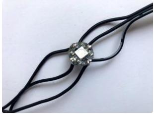
Measure out the length of wire you want. Cut it to length. If you're using just one NeoPixel, solder the striped wire to +, the middle wire to IN, and the third wire to G.
