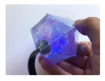
Slip each pixel inside the end of your crystal and secure it in place with hot glue. Add your crumpled up cellophane diffuser, then secure the crystal's open flap with krazy glue.
