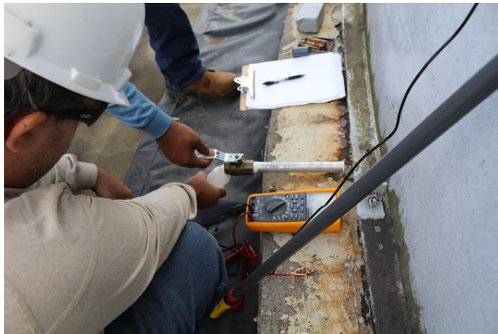
Figure 20: Photograph showing collection of liquid samples from the space between the tank bottoms of the storage tank.
