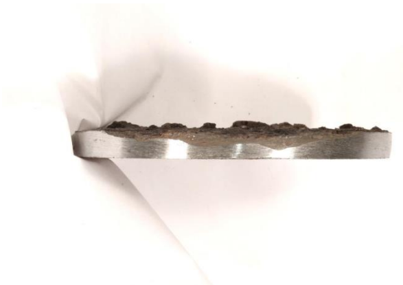
Figure 6: Photograph shows the locations of maximum corrosion product thickness and loss of thickness due to corrosion.
