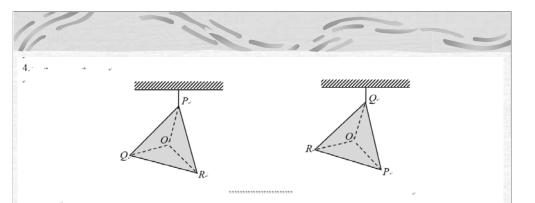
O is the centre of a metal plate PQR in the form of an equilateral triangle with **non-uniform** mass distribution. The plate is suspended from the ceiling at P and then at Q as shown. The centre of gravity of the metal plate is-
