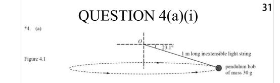
A pendulum bob of mass 30 g is tied to a fixed point *O* by a 1 m long inextensible light string. It is swirled to describe a horizontal circle uniformly at an angular velocity of 5.0 rad s<sup>-1</sup> as shown in Figure 4.1. Neglect air resistance. ( $g = 9.81 \text{ m s}^{-2}$ )
