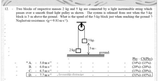
Over 30% of the candidates just considered the 5 kg block as a free falling object and arrived at the incorrect option D.-
