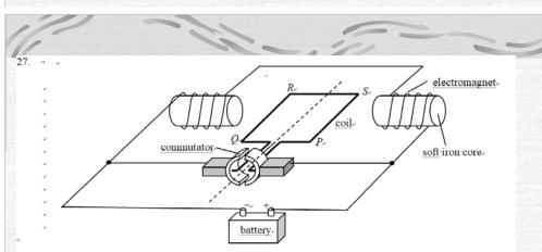
The figure shows the structure of a motor. The coil *PQRS* and the two electromagnets are connected to a battery so that the coil rotates continuously. If a sinusoidal a.c. source of frequency 50 Hz is used instead of a battery, the coil will-
