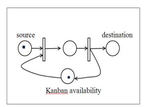
Fig. 17 Work-in-Process control sub-pattern
