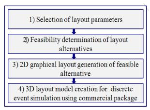
Fig. 5 Proposed procedure for FMS layout design
