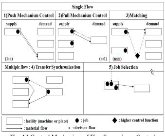
Fig. 14 Control Mechanism of Five Supervisory Control Patterns
