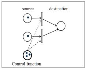
Fig. 18 Supply selection control sub-pattern
