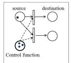
Fig. 16 Destination selection control sub-pattern
