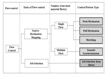
Fig. 13 Tasks of Flow Control
