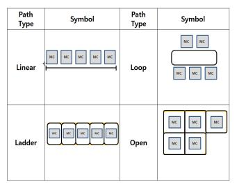
Fig. 3 Transport path type of FMS
