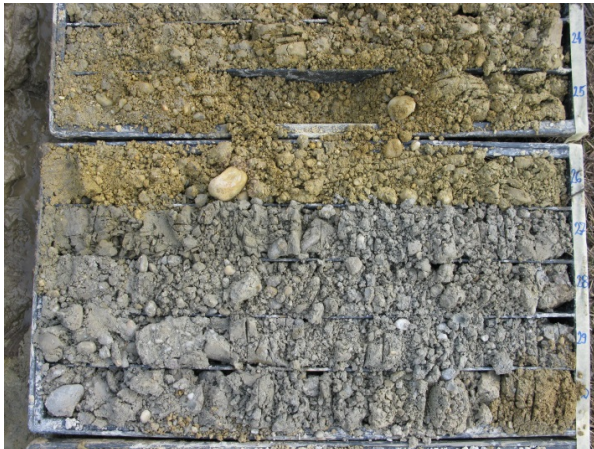
Figure 10. Gravel borehole core from 23 to 30 m depth et borehole SPB-3 (see Fig. 9).
