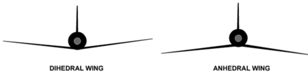
Figure 41: Dihedral and Anhedral Wing on Aircrafts
