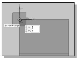
3. Use the **Profile** command and start the first line segment at the top left corner as shown.
