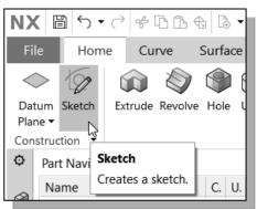
This toolbar contains tools that allow us to quickly access Datum features and switch to Sketch options.
