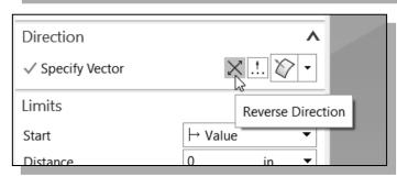
9. In the Direction option box, use the **Reverse Direction** icon to toggle the extrusion direction so that the extrusion cut through the bottom section of the model.
