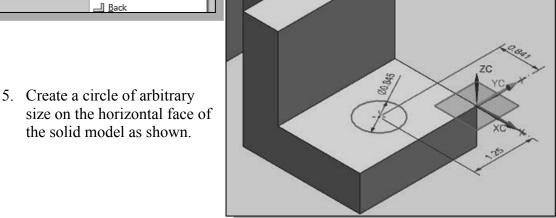
6. On your own, modify the dimensions of the sketch as shown in the figure. (Hint: there are two locational dimensions and one size dimension.)
