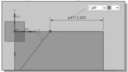
9. Select the two line segments and place the angular dimension inside the triangle to create the associated angle dimension.
