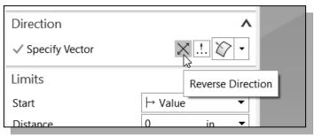
13. In the Direction option box, use the **Reverse Direction** icon to toggle the extrusion direction so that the extrusion cut through the bottom section of the model.
