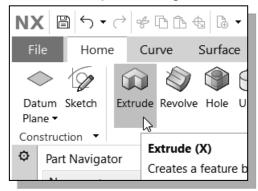
1. In the *Feature Toolbar* (toolbar next to the *Sketch* toolbar in the *Ribbon Bar*), select the **Extrude** icon as shown.
