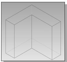
**❖** Wireframe with Dim Edges
