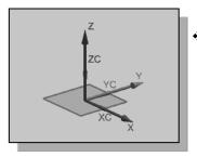
❖ Note the default sketch plane is aligned to **the XC-YC plane** of the displayed *Work Coordinate System*.
