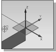
Note that the sketch plane is aligned to the selected face. Siemens NX automatically establishes a Work-Coordinate-System (WCS) and records its location with respect to the part on which it was created. 3. Select the **Circle** command by clicking once with the **left-mouse-button (MB1)** on the icon in the *Sketch Curve* toolbar.
