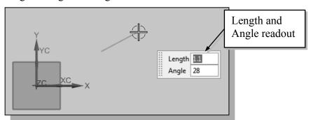
4. Move the graphics cursor directly above the previous point and create a vertical line as shown below (**Point 2**). Notice the geometric constraint symbol displayed.
