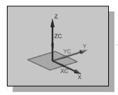
❖ The default sketch plane is aligned to the XY plane of the Work Coordinate System.
