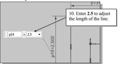
❖ When two parallel lines are selected, the Rapid Dimension command will create a dimension measuring the distance between them.
