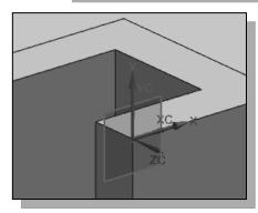
Note that the sketch plane is aligned to one of the corners of the selected face. *Siemens NX* automatically establishes a *Work-Coordinate-System* (WCS) and records its location with respect to the part on which it was created.
