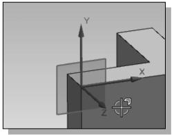
Note that the sketch plane is aligned to the selected face. *Siemens NX* automatically establishes a Work-Coordinate-System (WCS) and records its location with respect to the part on which it was created.
