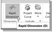
Activate the **Rapid Dimension** command by leftclick once on the icon as shown. The **Rapid** Dimension command allows us to quickly create and modify dimensions. 3. The message "Select object to Dimension or select dimension to edit" is displayed in the Message area. Select the **Top horizontal line** by left-clicking once on the line.
