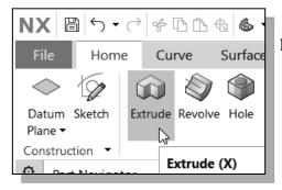
1. In the *Feature Toolbar* (toolbar next to the *Sketch* toolbar in the *Ribbon Bar*), select the **Extrude** icon as shown.
