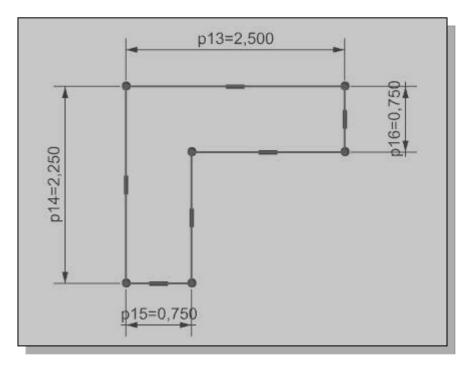
❖ The Rapid Dimension command is also known as the Smart Dimension command; dimensions are created based on the selection of the types and orientations of objects. You might want to read through this section again and consider the powerful implication of this command. Also consider this question: How would you create an Angle dimension using the Rapid Dimension command?
