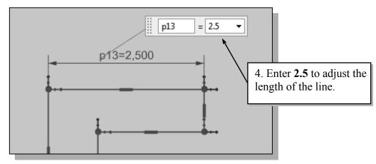
> Siemens NX will now update the profile with the new dimension value. Note that in parametric modeling, dimensions are used as **control variables**.
