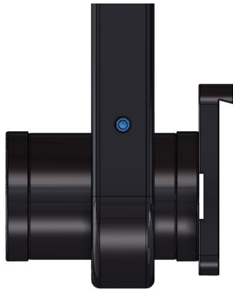
Figure 46: Location of the clamp setscrew on the bottom of the fork arm.
