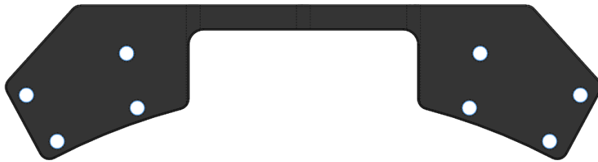
Figure 7: Eight 5/16-18 threaded holes for Officina Stellare 400 OTA bracket (front and rear are the same)
