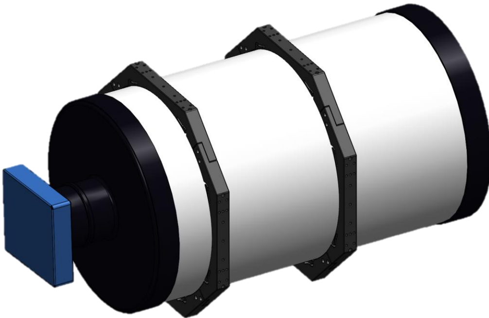
Figure 33: Meade 16-inch with two OTA mounting rings attached.
