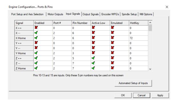
In the Config dropdown menu, the Operator can click Ports and Pins, then click the Input Signals tab to view input signals for all Axes as well as E-stop.
