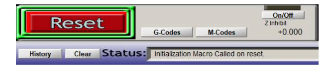
However, if the Operator needs to jog the machine, it can be accomplished by going into Mach3 and clicking Reset, then clicking Reset a second time.
