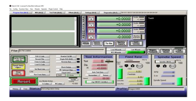
When powering up the Dragon A400 and its operational software, it is critical to follow the correct order of operations. The Operator may encounter a situation where Mach3 was minimized on the computer screen and the machine was shut down without closing out of Mach3. If the machine is re-started with Mach3 still open, a number of connectivity-associated error messages and problems will occur.
