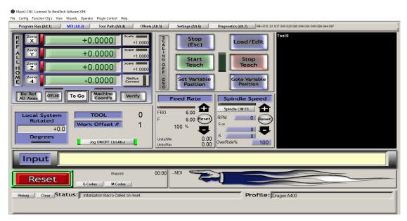
In the Input text box the Operator can enter an M code to tell the machine to perform an operation. For example, if there is a problem with the Torch, the Operator can enter the M code to fire the Torch to determine if it is a problem with the plasma unit, the machine or software.
