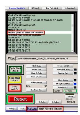
In the G-code display, click the up arrow on the right-hand side of the display twice to move the command line back two steps in the code. This is the command to lower the Torch to the cutting position.
