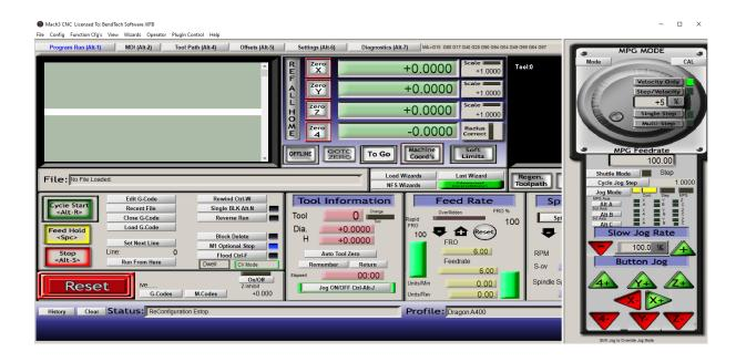
The Operator can access jog controls within any Mach3 interface by pressing the Tab button on the keyboard. The Operator can jog the X, Y, Z and A Axes within Mach3. Press the Tab key again to close out of the jog control interface.
