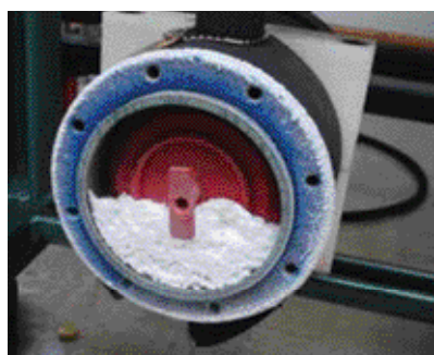
⤴ Figure 4 Example of dry ice formation in a drier.
