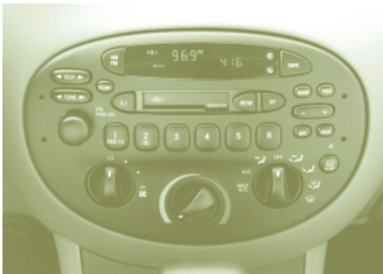
This film-insert-molded control panel has a decorative matte finish with backlit figures and symbols.
