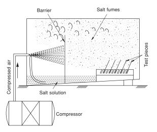
Figure A13.9 Salt spray chamber
