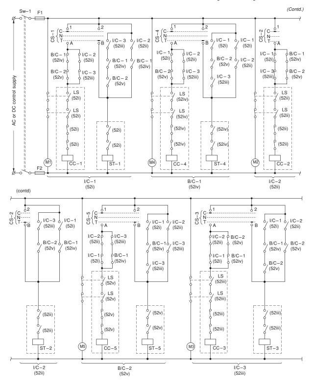
Figure 13.47 Control scheme for three electrically operated breakers, two bus couplers and three sources of supplies
