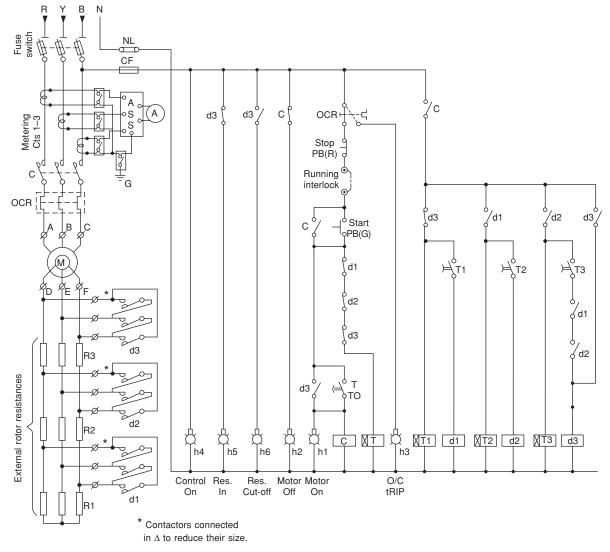
Figure 13.60 Typical three-stage stator-rotor starter
