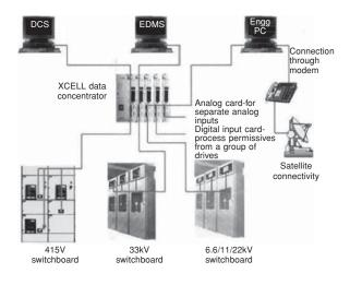
Figure 13.9(c) Application of intelligent switchboards for remote monitoring and control for total power automation (Courtesy: Larsen & Toubro)
