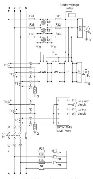
Figure 13.62 Schematic for instruments' wiring
