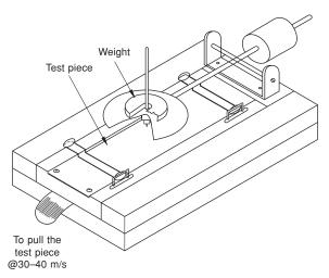
Figure A13.7 Scratch hardness testing apparatus
