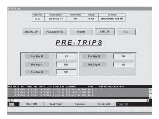
Figure 13.9(h) Typical display of pre-trip values (Courtesy: L&T)
