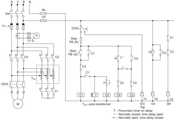
Figure 13.57(a) Auto-transfomer starter using pneumatic timer
