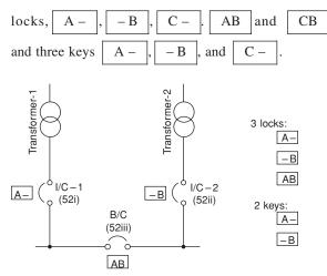
Figure 13.40 Two sources of supply and a bus coupler
