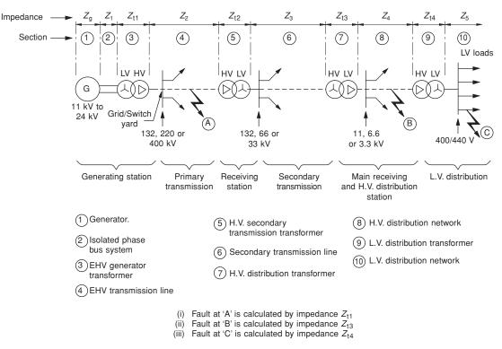
Note The actual fault at any point will be much lower than calculated with the above impedances  $Z_{11}$ ,  $Z_{12}$ ,  $Z_{13}$  and  $Z_{14}$  because other impedances from the source of supply (Transformers in the above case) up to the point of fault, are not considered while designing a system.
