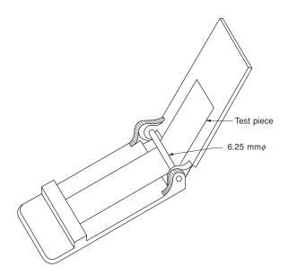
Figure A13.6 Apparatus for determining flexibility and adhesion
