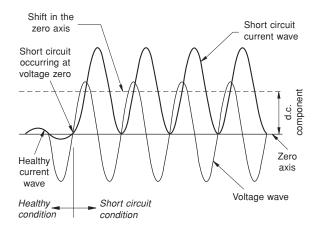
**Figure 13.26** Illustrating a shift of nearly 90° (drawn at 90° for ease of illustration) in the current wave at nearly 0.1 PF, fulfilling the condition of current lagging the voltage by nearly 90° yet rising together at zero voltage (minimum applied voltage)
