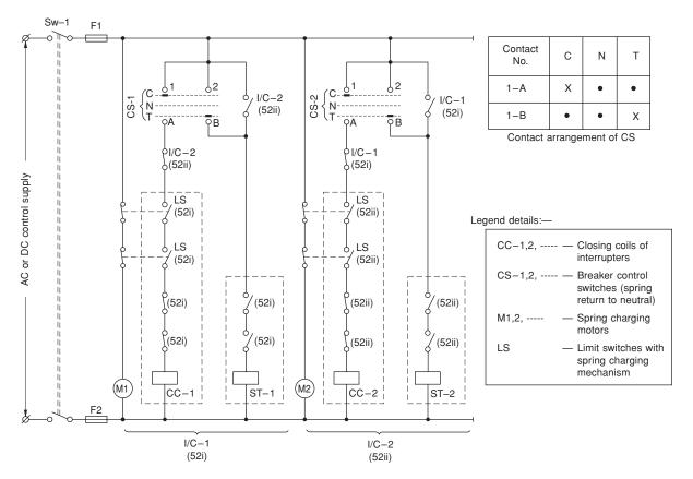
Figure 13.45 Control scheme for two electrically operated breakers and two sources of supplies
