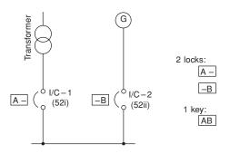
Figure 13.39 Two sources of supply
