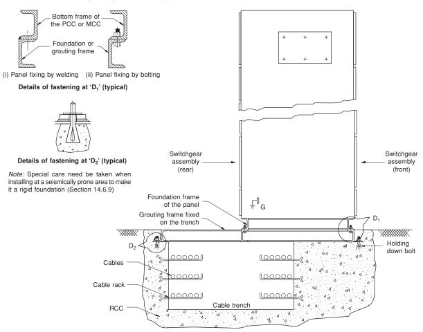
Figure 13.48(a) Illustration of a typical installation of high-rating switchgear assembly on a cable trench
