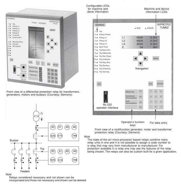
Figure 13.47(c) Typical feeder protection and views of a few relays
