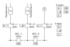
Figure 13.41 Three sources of supply and two bus couplers (Figures 13.39–13.41 are mechanical interlocking schemes)
