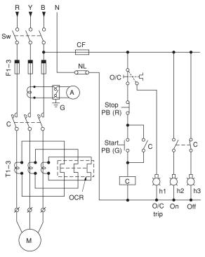
Figure 13.54 DOL starter with CT-operated over-current relay (i) For a high-rating motor or
