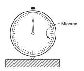
Figure A13.8 Thickness tester gauge
