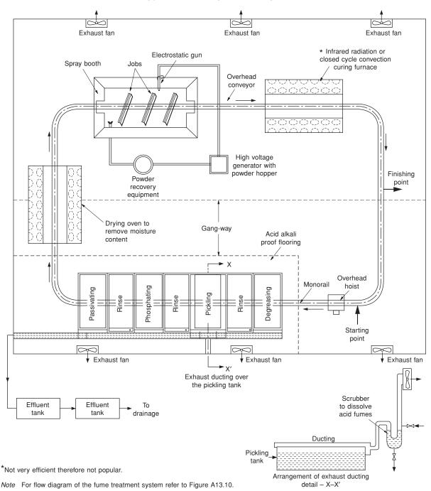
Figure A13.4 A dry painting system illustrating typical layout of a medium-sized paint shop for powder painting showing a seven-tank pre-treatment process
