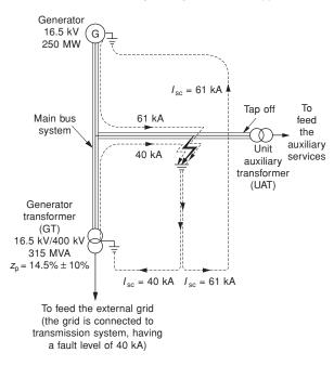
Figure 13.18 Fault level of tap-offs of a bus system under cumulative influence of two power sources
