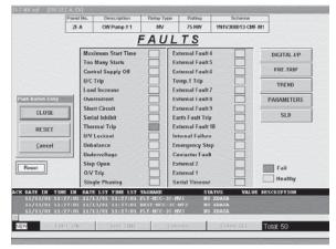
Figure 13.9(d) Typical display of faults (Courtesy: L&T)
