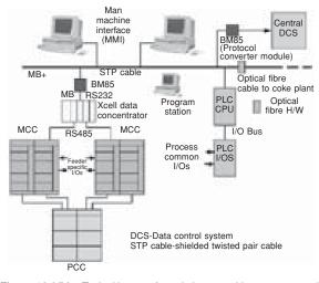
Figure 13.9(b) Typical layout of a switch room with remote control station at Tata Steel (Courtesy: Larsen & Toubro)
