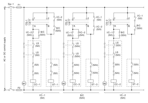
Figure 13.46 Control scheme for two electrically operated breakers, a bus coupler and two sources of supplies
