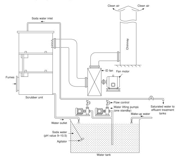
Figure A13.10 Typical flow diagram for fume treatment system
