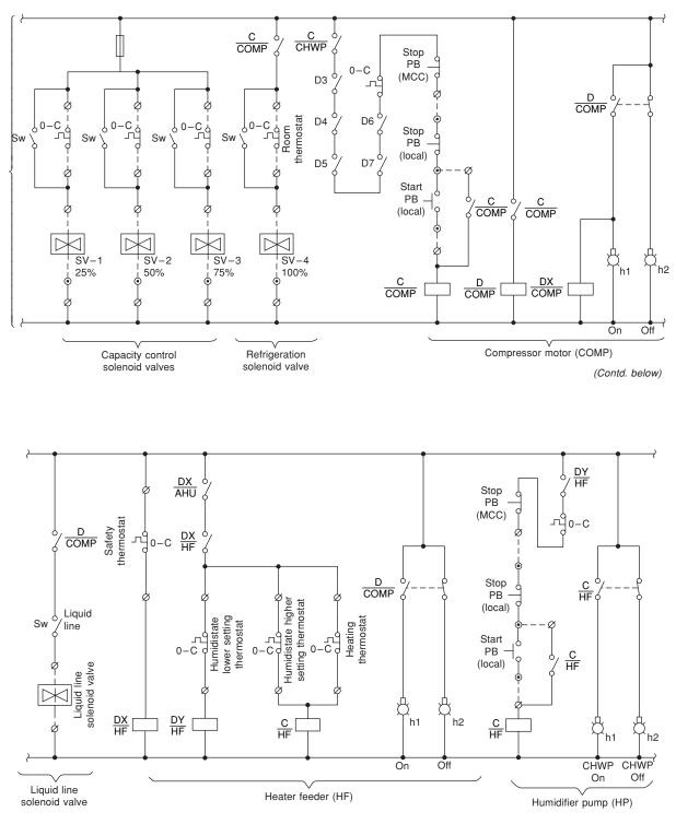
Figure 13.51 Control, protection and interlocking scheme for the air conditioning plant of Figure 13.50
