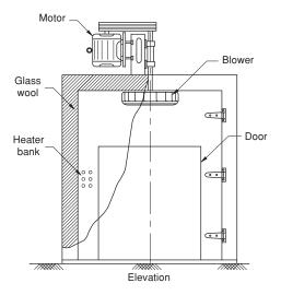
Figure A13.2 Closed-chamber convection-type furnace
