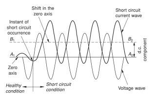
**Figure 13.27** Approximate illustration of a short-circuit condition occurring when both voltage and current waves are not at their natural zeros. Current shifting its zero axis from  $A_1 A_2$  to  $B_1 B_2$  to rise from zero again at the instant of short-circuit
