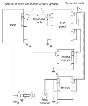
*Note* It is recommended to provide isolated grounding system for electronic circuits (see Section 6.13.3).
