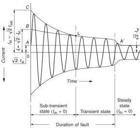
Symmetrical fault current at  $V_{\text{max}}$ , when  $I_{\text{dc}} = 0$
