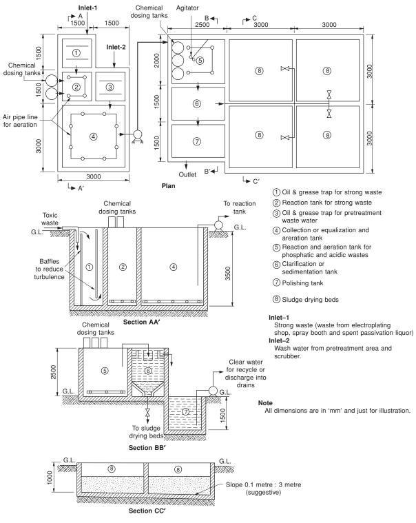
Figure A13.12 Layout of a typical effluent-treatment plant
