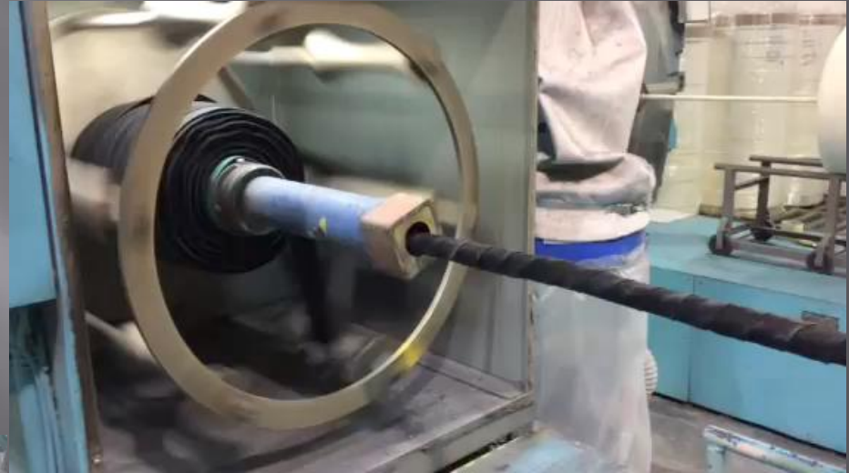
Wrapping of Aerogel over Mylar
