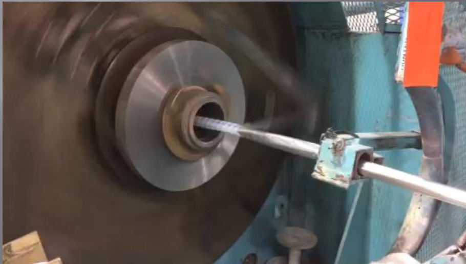
Wrapping of aluminum Mylar over Cabled tubes and heater
