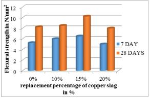
Fig.7. Comparison of Flexural Strength of Beam
