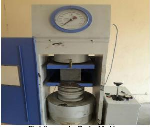
Fig.1.Compression Testing Machine
