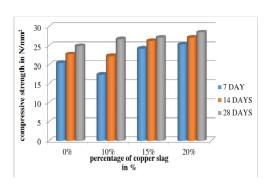
Fig.2.Comparison of Compressive Strength of Cubes
