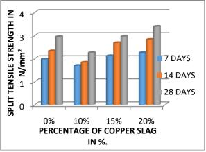
Fig.4.Comparison of Split Tensile Strength of Cylinders
