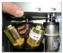
Figure 43. Use the Wheel to Raise and Lower Solenoid Manifold
