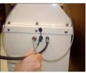
Figure 24. Connection of Air Line to the Lower Stand (Pump Enclosure)
