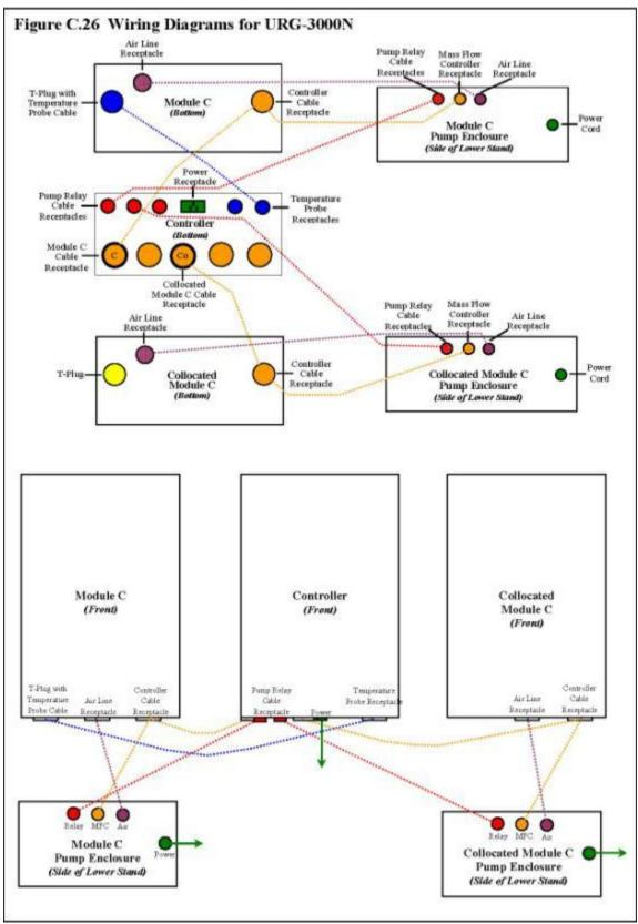
Figure 26. Wiring Diagrams for URG-3000N
