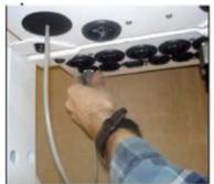
Figure 25. Connection of the Ambient Temperature Probe to the Sample Module and Controller Module
