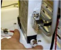
Figure 52. Removing MFC and Base Plate
