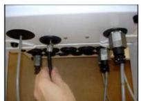
Figure 23. Connection of Air Line to the Sample Module
