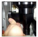
Figure 60. Unscrewing the Cyclone Ring
