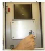
Figure 28. Inserting the Compact Flash Memory Card
