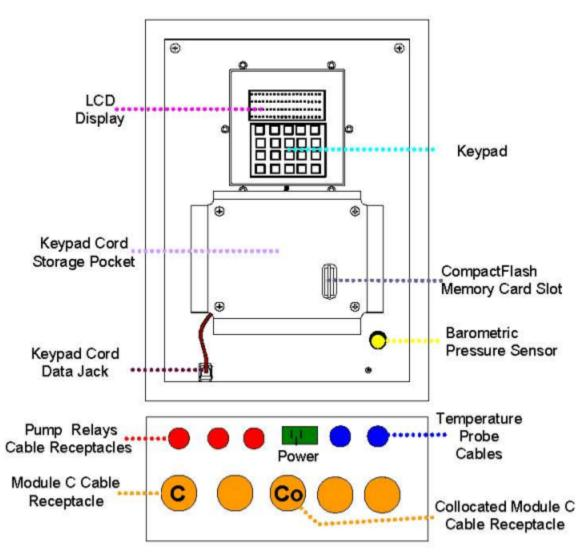
Figure 3. Controller Module
