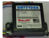
PN: W UHF2150A Whelen Headlight Flasher (Wig-Wag) w/ 4 flash patterns
