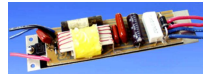
PN: TL IB-P116 TL IB-P112 Thin-Lite Ballast for lights with (2) F15T8CW bulbs, 30W
