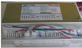
PN: W UPS158A Whelen Strobe Power Supply, 8 Outlet, 158 Watt
