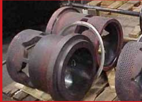
Fisher® 20" EHD Plug & Stem Assembly with Cage
