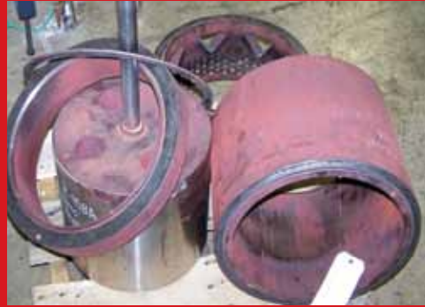
Copes-Vulcan® 12" Plug & Stem, Seat Ring, Cylinder Assemble & Balance Cylinder
