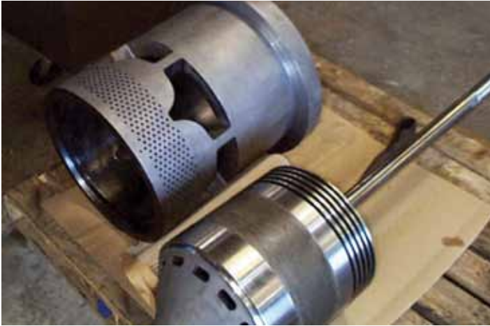
Fisher® 20" EHD Plug & Stem Assembly, Seat Ring & Cage
