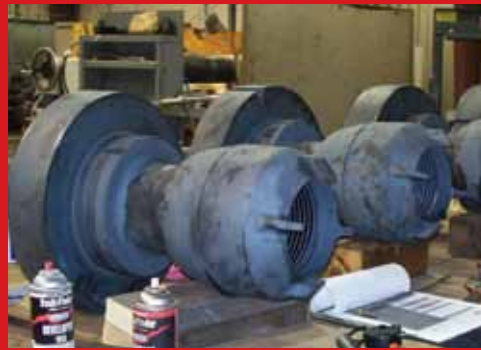
Siemens® HP Main Control Valve Bonnet with Spindle and Bushings
