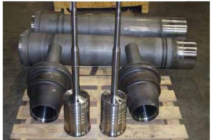
Alstom® High Pressure Spindles, Locks & Seat Chambers
