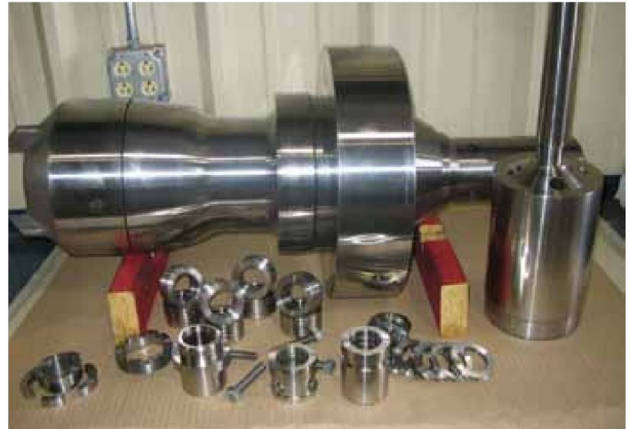
Siemens® High Pressure Main Control Valve Bonnet with Spindle & Bushings
