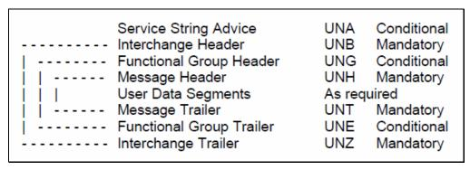
Figure 1 - EDIFACT Interchange Structure
