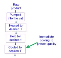
Fig. 5.1 Basic operations in a vat pasteuriser
