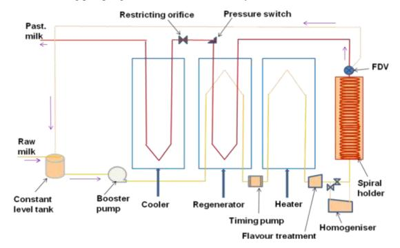
• Here the timing pump regulates the flow rate of the system at all the times.
