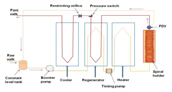
Fig. 5.7 HTST pasteurization process
