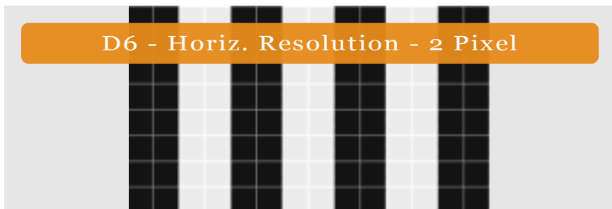
The original unscaled video contains two pixel wide columns that alternate between black and white.
