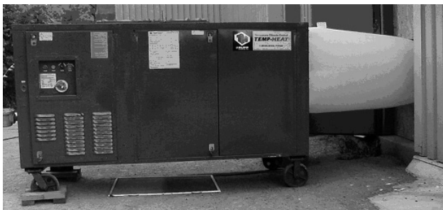
Figure 3. Propane-fired heater (Temp-Air) heater (source of heat for studies in Figure 2). The door is sealed with plywood, and a flexible fabric duct delivers heated air through a hole cut in the plywood.
