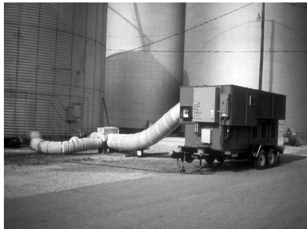
Figure 1. Grain chillers (From Burks et al. 2000).
