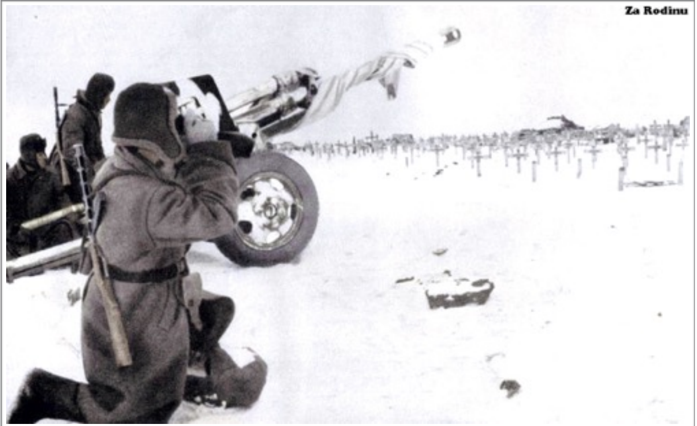
Soviet artillerymen firing a 76mm divisional gun M1942 (ZIS-3) during the Battle of Stalingrad.
