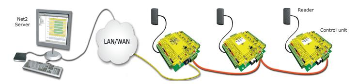
The data line must be wired in a single daisy chain. The data converter may be located anywhere along the data line. 120 ohm terminating resistors must be linked across each data pair at the beginning AND end of the line. This can be done on many units with a switch or jumpers. If not, free resistors are provided with the converter.
