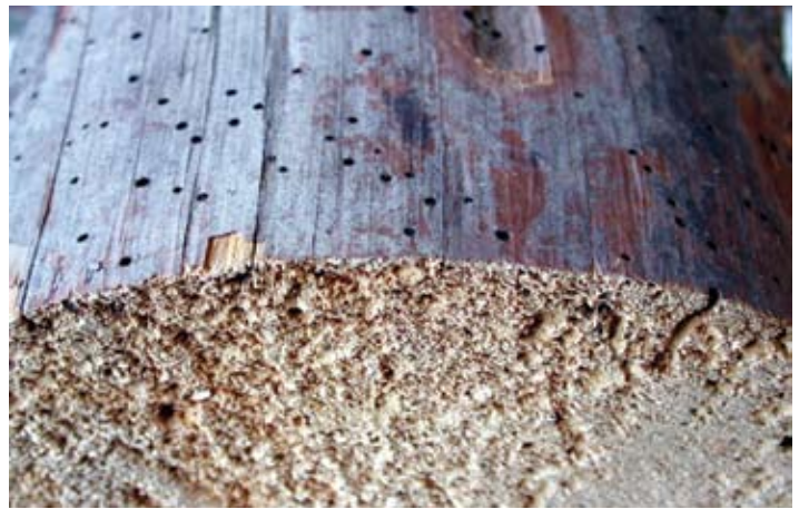
The surface of this log has numerous powderpost beetle entry holes. Powderpost beetles can attack and re-infest logs after they are assembled into a home.
