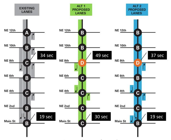
Note: PM peak hour intersection level of service (seconds/vehicle).
