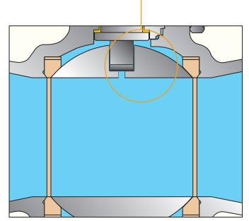
PBV® Valve's Series 4400/6400/5400/4500/6500 valves have all been proven to be Firesafe to API 607 or API 6FA. As illustrated, full metal-to-metal contact is attained at all sealing areas after the primary soft seals have been destroyed during a fire.
