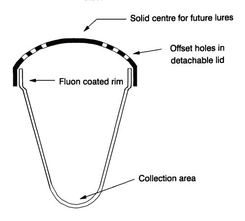
FIGURE 1. CROSS SECTION OF A PC TRAP.
