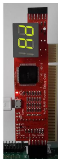
This shows using the large LPC connector on the other side of the diagnostic card to install on the motherboard that comes with the 2.54 large pin gap LPC connector. The dual side codes display design help to show the diagnostic codes clearly.
