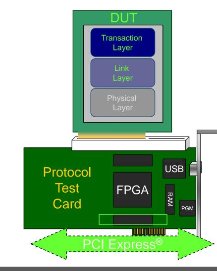
Test Control software running on platform or Device Under Test (DUT) initiates test traffic
