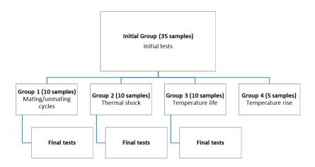
All testing was conducted per the relevant sections of AS39029D and any other industry standard document referenced within the specification.
