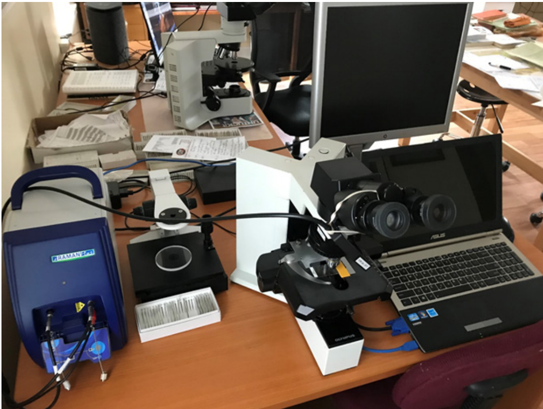
Figure 2. Photograph of the B&W Tek i-Raman Plus Raman system (left) interfaced with an Olympus polarizing microscope (center) as described in the text. Desk is 48 inches wide.
