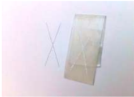
Method A - X-Cut Test and Adhesion Tape
