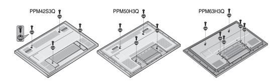
4 Put the 4 pegs on the PDP in the grooves of the wall mount bracket and pull down on the PDP (①) to secure it to the wall mount bracket (②). Tighten the screws as shown (③) so that the PDP cannot be separated from wall mount bracket.
