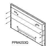
2 Hang the two "T" shaped hangers on the square holes on the rear of the PDP.
