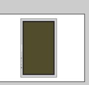
You can install the PDP vertically. (PPM42S3Q/50H3Q/63H3Q models are available. Other manufacturers do not guarantee a reliably working.) In this case, the fan automatically works. If you wish to stop the fan, position the PDP horizontally and then set "Selectable Fan" to "Off" in the "Function" menu.
