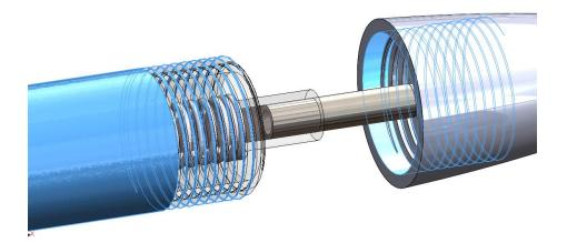
Add a **coincident mat**e between the end-points of the threads.
