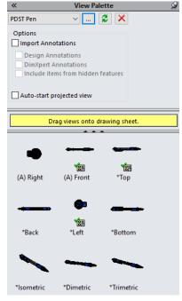
Drag the required view (Top) from the new **View Palette** onto the drawing sheet and edit the view
