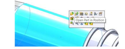
This part can also be opened separately by clicking on the part and selecting **Open Part in Position**.
