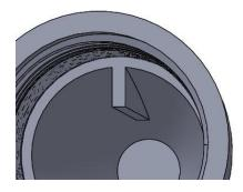
Using **Circular Pattern** complete the feature about the temporary axis as shown
