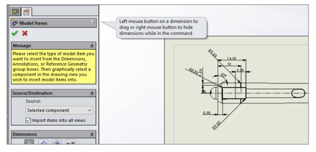
Select the Dimensions using the Lasso Right to Left and click the dimension palette rollover button. The dimension palette offers a number of adjustments that can be made to the dimension format.
