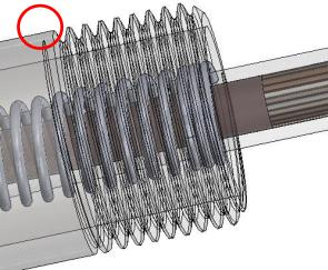
The endpoint of the thread on the body will be difficult to select because of the transparent appearance. The pen body must be rotated into a position where the end of the thread is at the edge and there is nothing else behind the point.
