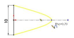
As the curser is moved along the construction line the Rho value is seen to change.
