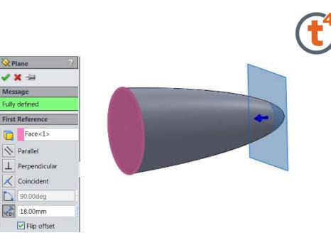
In the Surfaces commands select Cut With Surface and select the plane shown.
