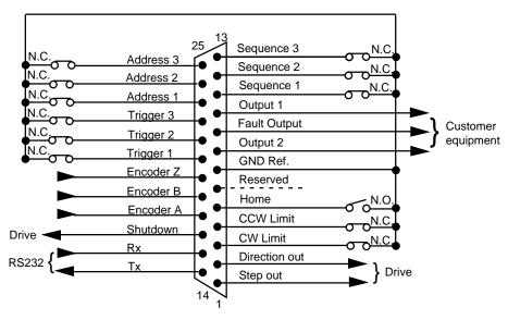
Figure 2 PDX Drive Indexer Connections
