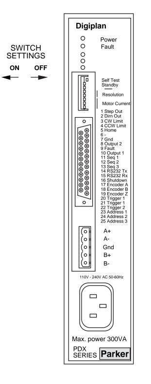
Figure 21. Front Panel Layout
