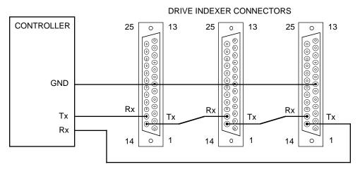
Figure 16 Daisy Chain Connection of Drives
