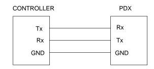
Figure 10 RS232 Connections
