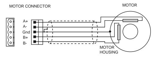
To reverse motor rotation relative to the direction input, interchange connections to A+ and A–.
