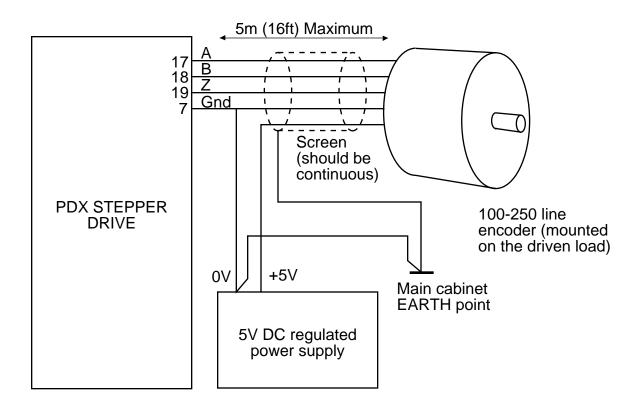
Figure 13 Wiring Example for PDX - Encoder Option
