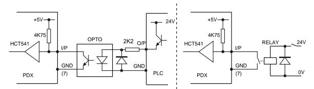
Figure 14 Trigger Input Example Connections
